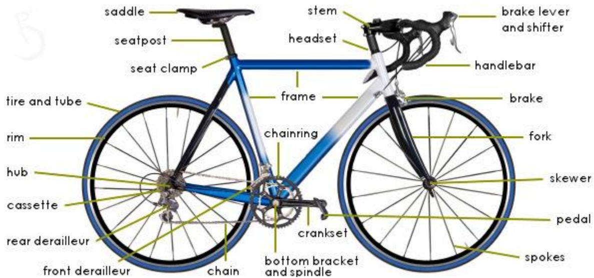
**Brake Lever** – Lever on the handlebars used to activate the brake caliper via a cable system.
